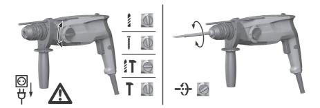
Set the function selector switch to the "Chisel positioning" position -9.
