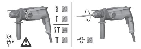
Set the function selector switch to the "Chiseling" position T.
