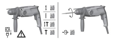
► Set the function selector switch to the "Drilling with hammering action" (hammer drilling) position (1.7).
