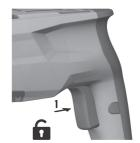
Press and lock the control switch.
