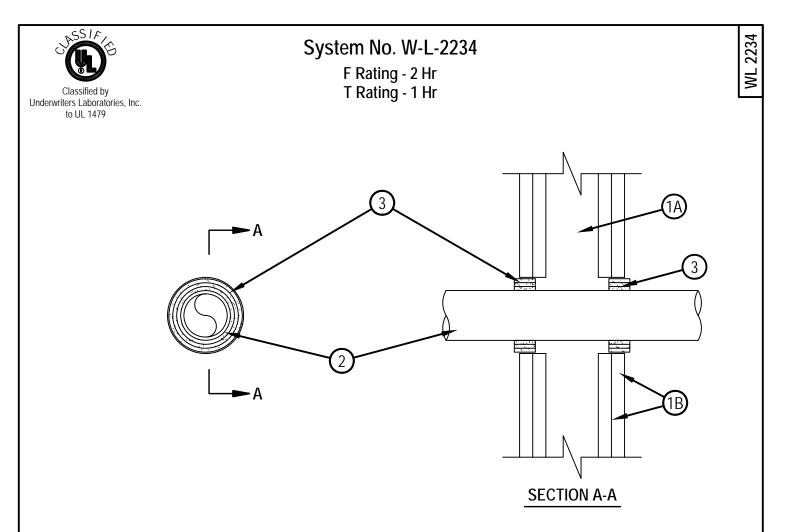
1. Wall Assembly -- The fire-rated gypsum wallboard/stud wall assembly shall be constructed of the materials and in the manner specified in the individual U300 or U400 Series Wall and Partition Designs in the UL Fire Resistance Directory and shall include the following construction features:
