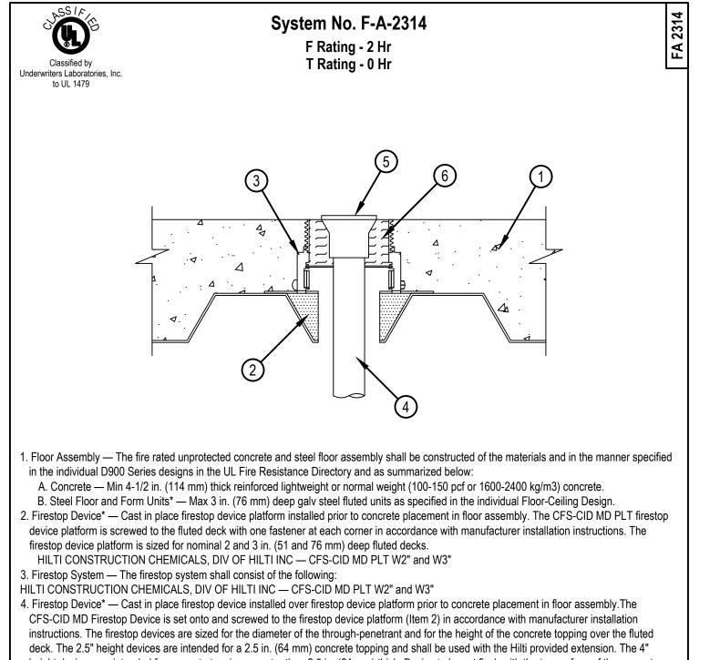
height devices are intended for concrete toppings greater than 2.5 in. (64 mm) thick. Device to be cut flush with the top surface of the concrete. HILTI CONSTRUCTION CHEMICALS, DIV OF HILTI INC — CFS-CID MD P 2"/2.5", 3"/2.5" and 4"/2.5"; CFS-CID MD P 2"/4", 3"/4" and 4"/4", CFS-CID MD PX 2"/2.5", 3"/2.5" and 4"/2.5" and 4"/2" and 4"/4"
