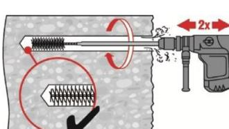
Screw the round steel brush Hilti HIT-RB in one end of the brush extension(s) HIT-RBS, so that the overall length of the brush is sufficient to reach the base of the drill hole. Attach the other end of the extension to the TE-C/TE-Y chuck.
