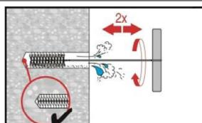
Brush 2 times with the specified brush (see Table B4) by inserting the steel brush Hilti HIT-RB to the back of the hole (if needed with extension) in a twisting motion and removing it.
