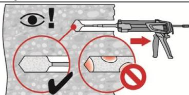
Inject the adhesive starting at the back of the hole, slowly withdrawing the mixer with each trigger pull.
