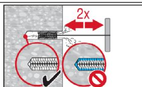
Brush 2 times with the specified brush size (brush  $\varnothing \geq$  drill hole  $\varnothing$ , see Table B4) by inserting the steel brush Hilti HIT-RB to the back of the hole (if needed with extension) in a twisting motion and removing it.
