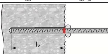
After installing the rebar the annular gap must be completely filled with mortar. Proper installation:
