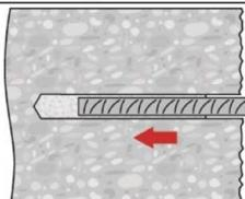
For easy installation insert the rebar into the drill hole while slowly twisting until the embedment mark is at the concrete surface level.
