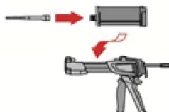
Tightly attach Hilti mixing nozzle HIT-RE-M to hard cartridge manifold. Do not modify the mixing nozzle.
