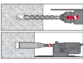
Drill hole to the required embedment depth with a hammer drill set in rotation-hammer mode, a compressed air drill using an appropriately sized carbide drill bit or a diamond coring machine.
