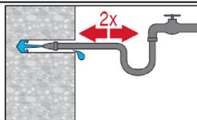
Flush 2 times by inserting a water hose (water-line pressure) to the back of the hole until water runs clear.
