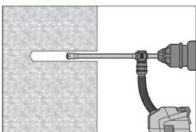
Drill hole to the required embedment depth with an appropriately sized Hilti TE-CD or TE-YD hollow drill bit attached to Hilti vacuum cleaner VC 20/40 (-Y) (suction volume  $\geq 57$  l/s) with automatic cleaning of the filter activated. This drilling system removes the dust and cleans the drill hole during drilling when used in accordance with the user's manual.
