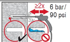
Blow again with compressed air 2 times until return air stream is free of noticeable dust and water.
