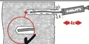
The Hilti hand pump may be used for blowing out drill holes up to diameters  $d_0 \leq 20$  mm and embedment depths up to  $h_{ef} \leq 10 \cdot \phi$ .
