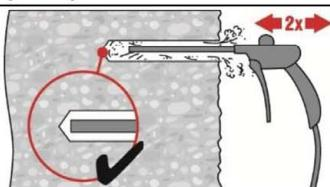
Blow 2 times from the back of the hole (if needed with nozzle extension) over the whole length with oil-free compressed air (min. 6 bar at 6 m<sup>3</sup>/h) until return air stream is free of noticeable dust.
