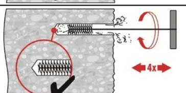
Brush 4 times with the specified brush (see Table B4) by inserting the steel brush Hilti HIT-RB to the back of the hole (if needed with extension) in a twisting motion and removing it.
