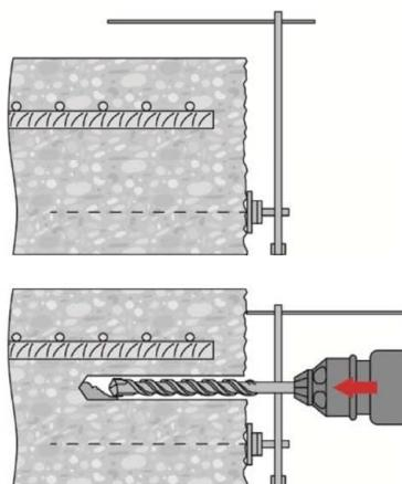
Ensure that the drill hole is parallel to the existing rebar.
