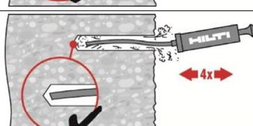
Blow out again with the Hilti hand pump at least 4 times until return air stream is free of noticeable dust.
