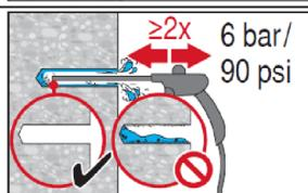
Blow 2 times from the back of the hole (if needed with nozzle extension) over the whole length with oil-free compressed air (min. 6 bar at 6 m³/h) until return air stream is free of noticeable dust and water.
