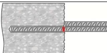
Observe the working time  $t_{work}$  (see Table B3), which varies according to temperature of base material. Minor adjustments to the rebar position may be performed during the working time.
