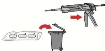
The hard cartridge opens automatically as dispensing is initiated. Prior to dispensing into the drill hole, squeeze out separately 3 full strokes.
