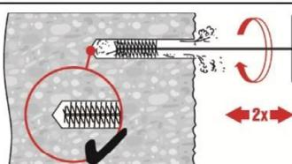
Brush 2 times with the specified brush (see Table B4) by inserting the steel brush Hilti HIT-RB to the back of the hole (if needed with extension) in a twisting motion and removing it.
