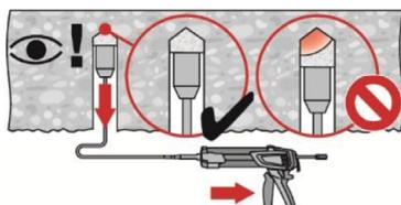
For overhead installation the injection is only possible with the aid of extensions and piston plugs. Assemble HIT-RE-M mixer, extension(s) and appropriately sized piston plug (see Table B4). Insert piston plug to back of the hole and inject adhesive. During injection the piston plug will be naturally extruded out of the drill hole by the adhesive pressure.
