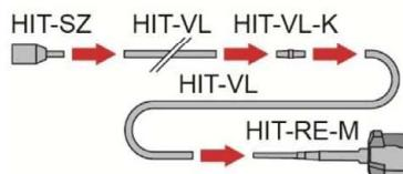
Assemble mixing nozzle HIT-RE-M, extension(s) and piston plug HIT-SZ (see Table B4).
